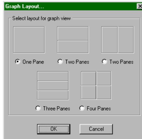
There are two ways to display multiple graphs in *Logger Pro*; one is to use two or more graph windows, and another is to use the Graph Layout command to display two or more graph panes within a single window. Graphs in separate windows are independent of one another, although both depend on the same data table. Graph panes in a single window share certain adjustments for ease of viewing. These shared parameters are:
