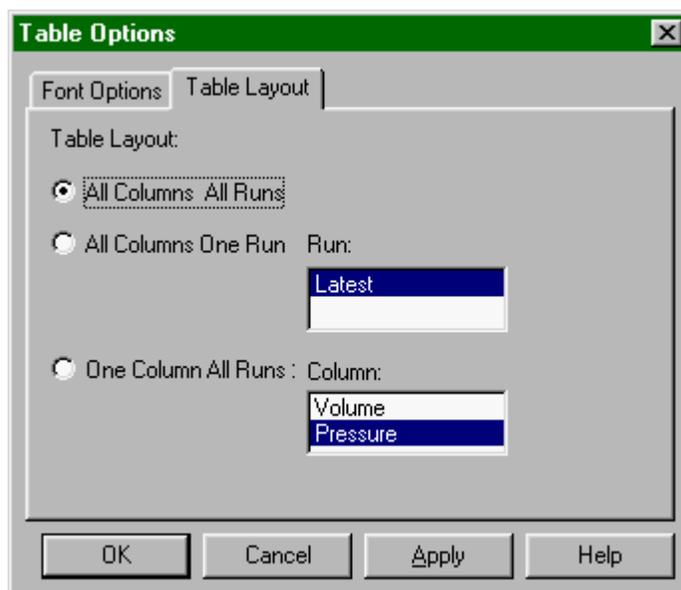
Choose the table layout you need. The choices allow you to display all columns from all runs, just a single run, or just one column from all runs. You can further control what is shown in the data table by hiding individual columns in the Column Options dialog found in the Data menu, or by double-clicking a column header.
