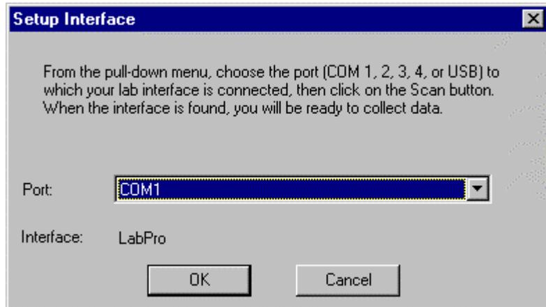
It is only necessary to use this dialog if *Logger Pro* is started without the interface connected or powered, or if communication with the interface is lost.
