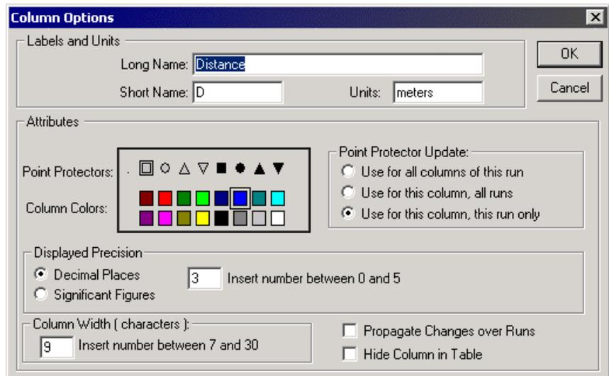
In the Column Options dialog you can change the column's name, color, decimal places displayed, and width. If you click in the box for Propagate Changes, all runs for that column will be affected. Hide Columns will conceal the column in the data table. You can choose to apply the new point protector to all columns of that run, all runs for that column, or that column and run only.
