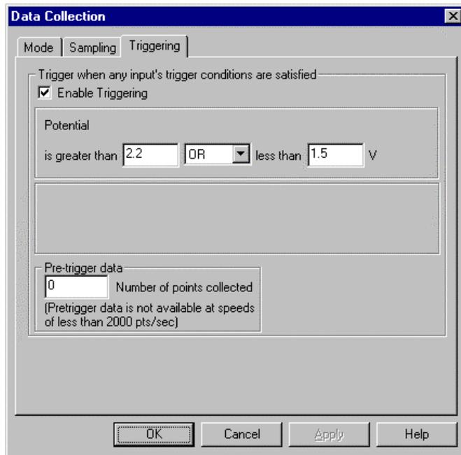
When using the LabPro interface and a fast rate data collection, the dialog is slightly different to account for the fact that LabPro uses edge triggering at these rates.
