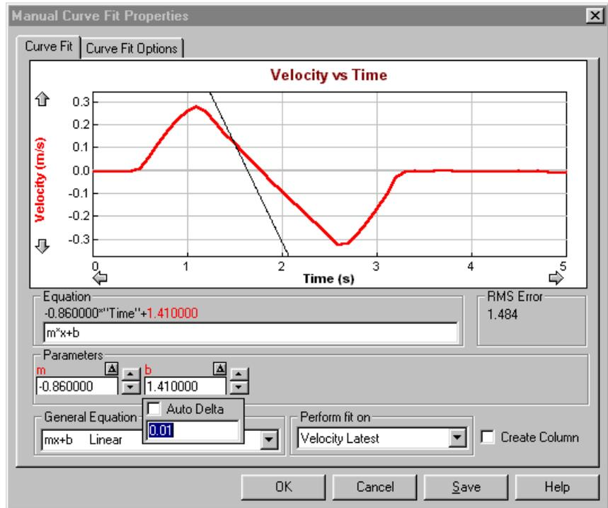
First, you must select or enter an equation. The faster method is to select an equation from the General Equation menu. In the screen shown above, the linear relation  $y = mx + b$  has been selected. You can also enter your own relationship in the Equation field. The equation must contain between one and five adjustable parameters (single upper- or lower-case letters) and the horizontal axis variable is entered as  $x$ .
