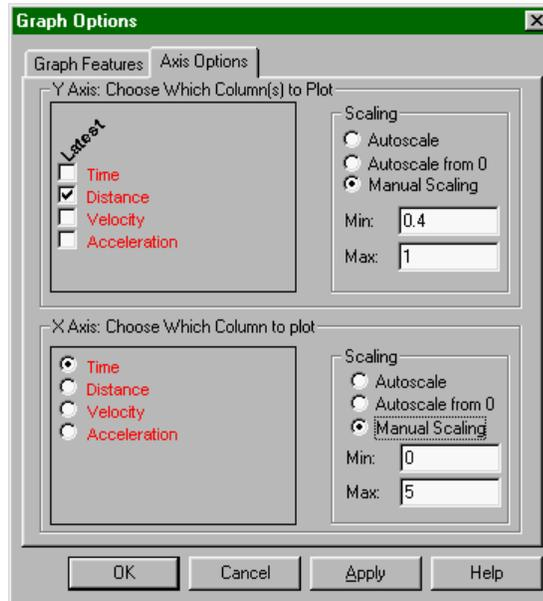
Here you can control what is plotted on the two axes as well as the scaling used. The settings here are duplicated in the axis scale and selection dialogs obtained by double-clicking an axis or axis label. The columns shown will depend on your specific configuration of *Logger Pro*. Scaling choices will also be used in subsequently collected data.
