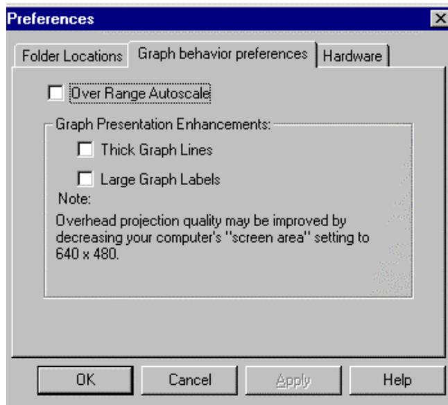
The Graph behavior preferences tab allows you to set graphing options. If Over Range Autoscale is checked, *Logger Pro* will automatically rescale the graph vertically during data acquisition to include any data point acquired even if it may exceed the existing range settings of the graph.
