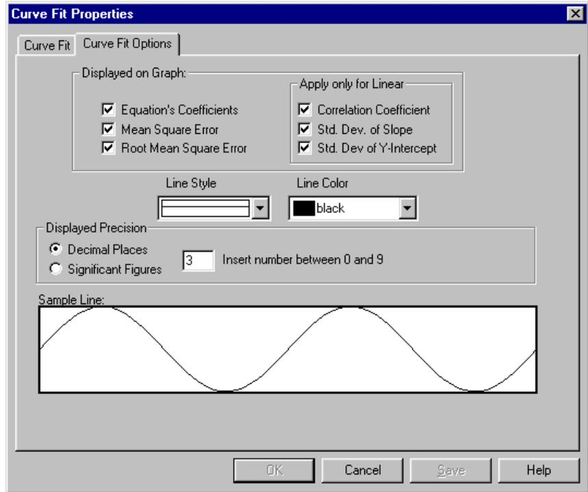
The Curve Fit Options tab allows you to determine which fit statistics are displayed on the graph. The Equation's Coefficients are the fitted parameters. The Mean Square Error and its square root, the Root Mean Square Error, measure how far away on average the fitted function is from the data. The Root Mean Square Error is in the units of the data on the y-axis.
