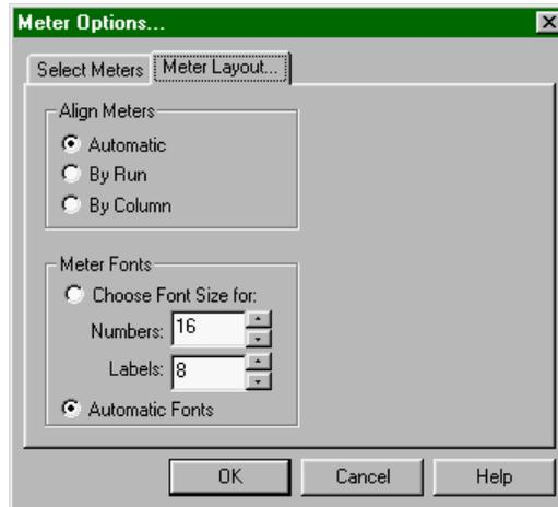
The three grid layout options determine whether the meters are laid out to fill the available space with the largest possible meters (Automatic), to arrange data from each run vertically (By Column) or horizontally (By Run).
