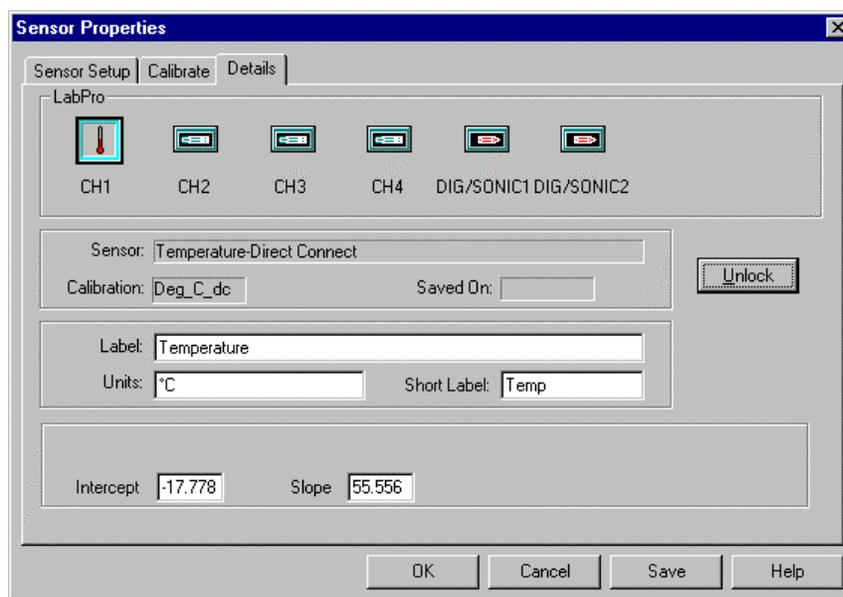
The calibration procedure creates a correspondence between the sensor voltage output and the measured quantity (such as temperature) which can be characterized by a slope and intercept. If someone has done an earlier calibration of a sensor you can manually enter the calibration here after clicking on the Unlock button. The Labels and Units can also be changed. For example, this is where you could enter the calibration parameters for a new sensor that does not have a supplied calibration file.
