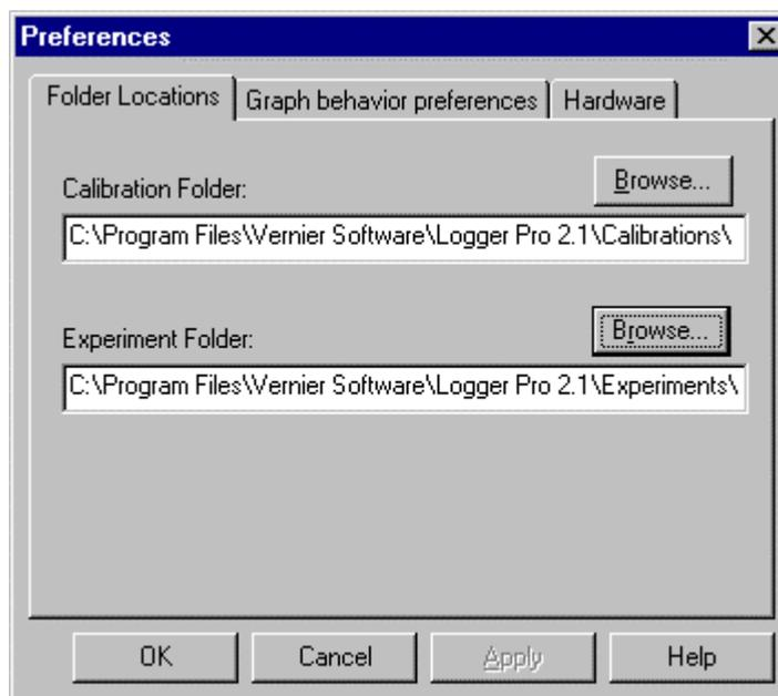
*Logger Pro* will only detect calibration files stored in the default calibration folder. New calibration files are saved to this folder as well, and will subsequently be available in the list of calibrations in the Sensor Setup dialog box.
