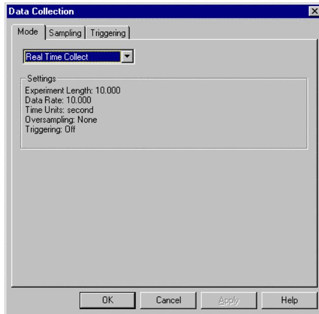
Select Real Time Collect from the scrolling list. In this mode data are collected continuously at the rate indicated and for the time interval set on the Sampling tab. To modify these settings, click on the Sampling tab.
